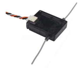
I am unclear whether the two "whiskers" on these devices are separate antennae or two parts of a dipole but the unit should be considered as a single antennae and oriented with the wires sticking out as in the picture and at right angles to those on the primary receiver.
