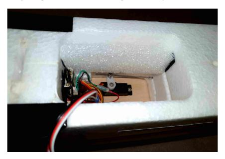
A small piece of self adhesive velcro "hook" material on the right hand side of the picture helps to keep the foam in place.
