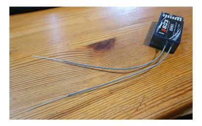
These are pieces of coaxial cable with about 30mm of the outer conductor stripped away at the end. The type and length of the cable and the amount stripped away may be matched to the type of receiver so if you damage an antenna get a proper replacement. The exposed "whisker" does the actual receiving.
