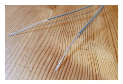
No installation is perfect, but our objective is to get the end bits straight, as far away from the rest of the receiver, wiring, servos or power installation as we reasonably can and, if possible, approximately at right angles to each other. The idea of having two antennae is that if the signal is poor in one it might be better on the other.
