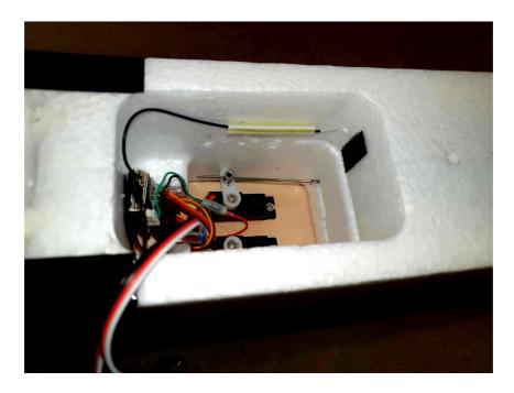
The picture above shows a piece of plastic straw holding an antenna in a Century Models Riot. The end of the "whisker" extends further into a hole I made in the expanded polystyrene. In this way the antenna is kept away from the wiring and the steel wire pushrods.
